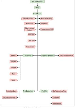
PV Module schema diagram
